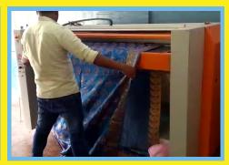
6 feet wide suitable for all type of cotton silk hand work sari with stone work Adjustable speed and temp with emergences stop trolley mounted for easy movement One touch micro controller For electrical model (12kw) size 6.5 feet x2.2feet
